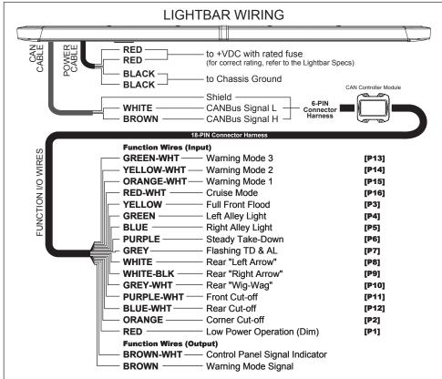
NOTE: All function wires (Input) are activated by applying +VDC continuously.
