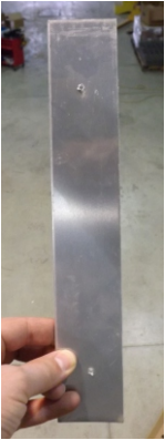
Example of an aluminum reinforcement (5cm x 30cm x 2.5mm)
