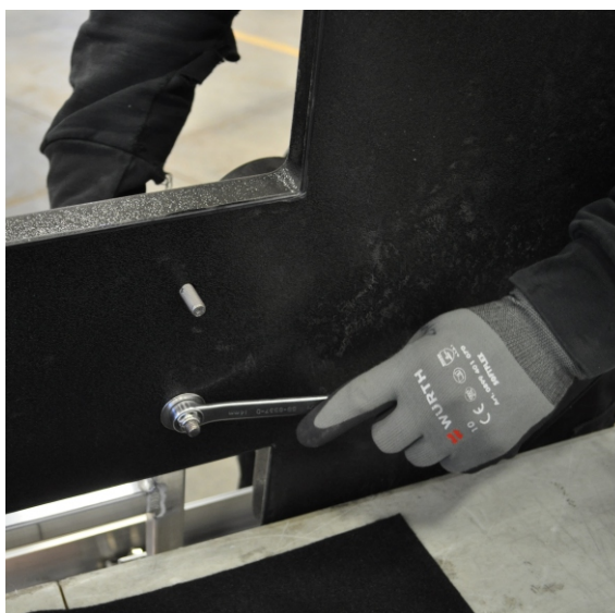
Make sure to put a washer on the front and back of the arrow for each bolt
